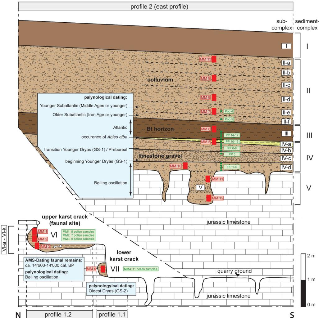
**Figure 3:** Schematic north-south profile with the lower (profile 1.1; VII) and the upper karst crack (P1.2; VI) and the east profile (profile 2) with another karst fissure (V) and colluvial deposits (I-IV). Sediment complexes and subcomplexes are given to the right. Red: soil monolith samples (micromorphology). Green: palynological samples. Dark brown layers: high content of clay. Yellow layers: calcareous loam. Drawing: David Brönnimann, based on Rentzel et al. 1999, Fig. 3.
