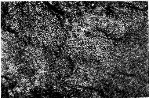
Fig. 5. Striations from grooving wood with low-angled edge using soft abrasive, 200x.
