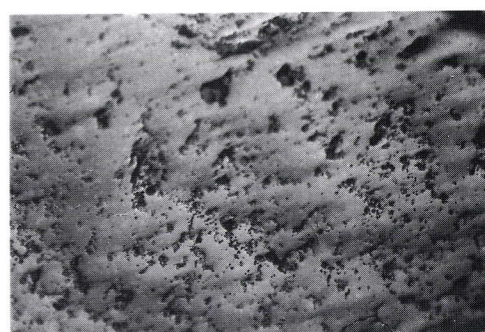
Fig. 29. Totally polished surface from buffing flint with 1/4 micron paste, 100x.
