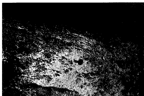
Fig. 38. B. Bright spot produced by rubbing flint on flint with water for 2 minutes (cf. fig. 38 : A), 200x.
