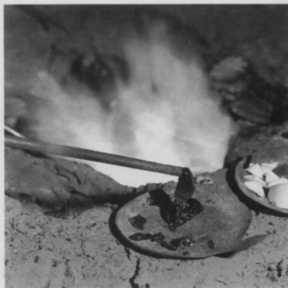
Fig. 10. How to make a gather : raw glass is preheated on the iron pan and melted directly on the pontil.
