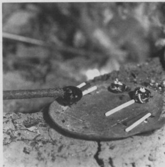
Fig. 8. Threadbands made by melting pre-heated rods of white and red glass on a small gather of blue glass.
