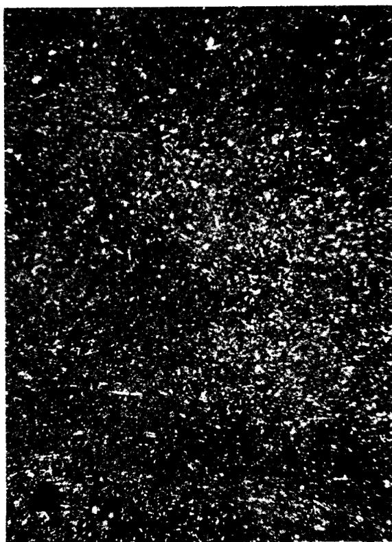
Fig. VII-9 Phot.5. Sample A-Ba-R1. Opal-chalcedony background with disseminated fine quartz. Polaroids X. 32x.
