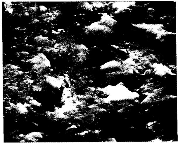
Fig. VII-14 Phot.25. Sample A-Gr-F2. Structural changes of the flint at zone of patination. Black internal part flint. Light patina. Between patina and internal part (arrow) one can see the zone of structural changes. SEM. 100x.
