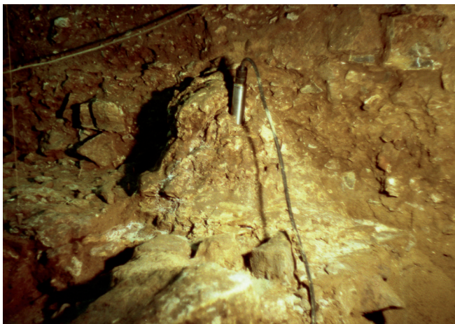
Figure 2. Measurement of gamma radiation intensity inside a large stalagmitic boss using a portable spectrometer. The stalagmite has been drilled with a coring machine, and a sample for TL dating has been obtained from the core. The detector of the spectrometer occupies the same position as the TL sample, and is recording gamma rays emanating from the stalagmite and underlying sediment.
