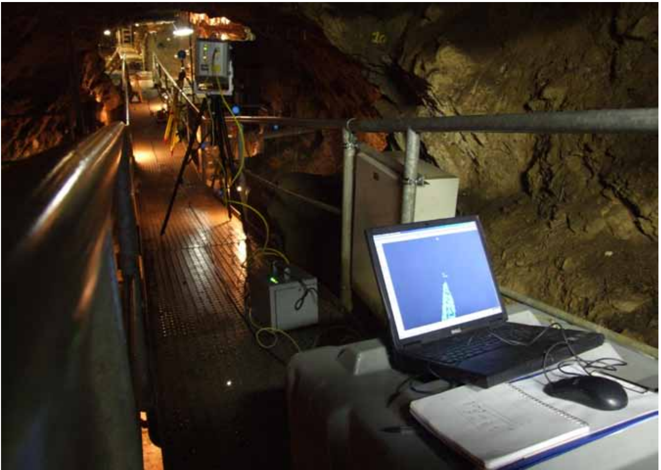
2008: with help from the State, a Cyrax 3D scanner records the inner morphology of Scladina Cave in high resolution.
