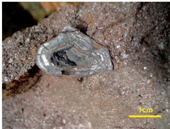
Fig. 11 – Emsian-Eifelian OIS, Heisdorf Formation, Hammermühle, Hillesheim (Germany). Large, ferruginized (hematitic) oncoïd, showing laminated texture. Fossil ore facies. Macroscopic view of rough surface. Scale bar is 1 cm.
