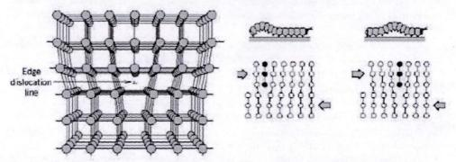
The first figure shows the meaning of torsion. In an otherwise perfect crystal, i.e. one free of inhomogeneities (in practice, difficult to achieve) an edge dislocation is produced, either by removal (i.e., introduction of singularities) of atoms of the crystal, as the figure shows, or by introducing extra material; thus, it is an action-dependent
