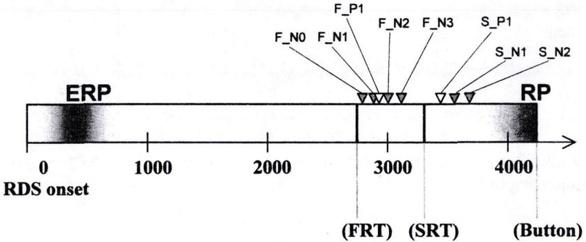
**Figure 14:** Time course relation of the ERP evoked by RDS/RDI presentation, brain potentials with referring to FRT and SRT, and RP evoked by button press in our experiment.
