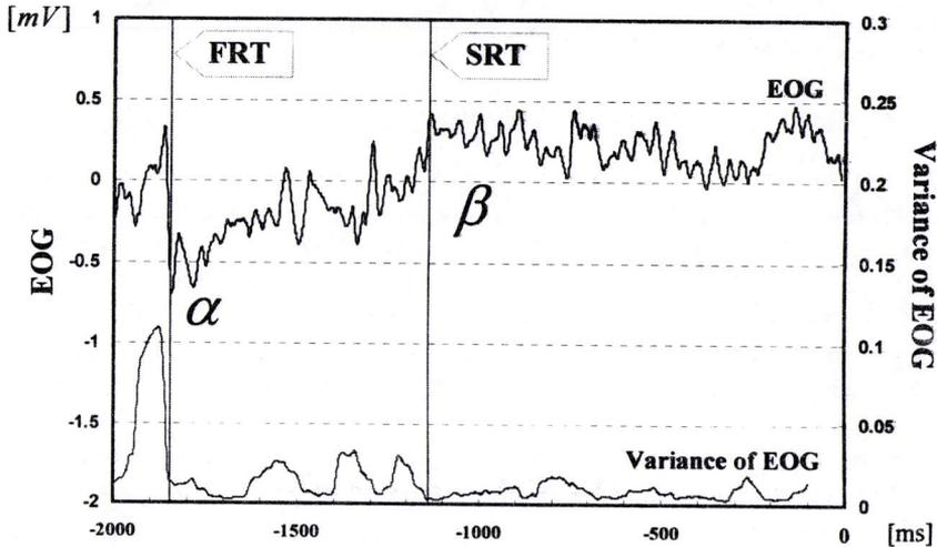
**Figure 5:** Typical profile of EOG (upper line) and the moving variance of EOG (lower line) 2000ms before the button press. EOG shows the rapid and discontinuous fluctuation ‘ $\alpha$ ’ and succeeding stable phase ‘ $\beta$ ’. Two reference times, “FRT” and “SRT”, were defined as described in the text.
