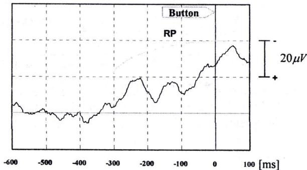
**Figure 12:** A typical readiness potential (RP) evoked by the button press. Negative modulation (RP) emerges from 300 ms before button press and 50 ms after that.
