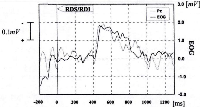
**Figure 15:** Example of the EEG profile at Pz contaminated with rapid eye movement shown as the fluctuation of EOG.
